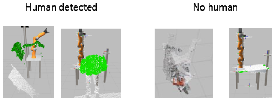
Figure 6. Octomaps detection: The octomap_binary occupancy grid is used to detecting human presence in the not allowed contact states .
